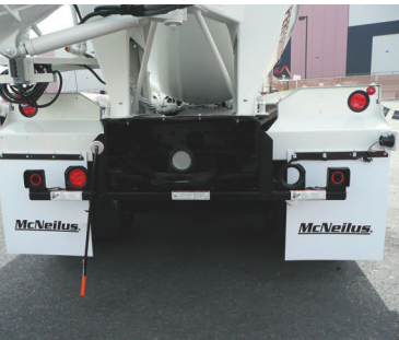
Can you see the defect? A tail light is missing — one of many “bugs” planted on this truck for the pre-trip inspection test.
