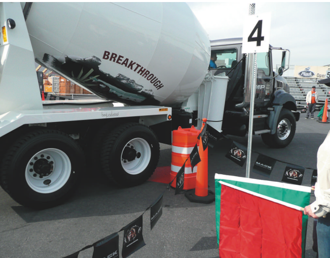
Above: Turning-radius test required the driver to go around the barrel while getting the right-rear wheels as close as possible without hitting it.
