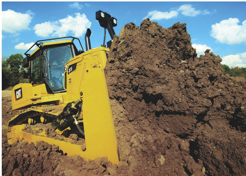
Electric drive is not the D7E's only innovation. A center-post cab broadens the view to each half of the blade, and oval track will replace the D7R's elevated sprocket.
