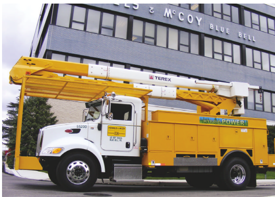
Hybrid basket trucks convert braking energy into stored battery power, and the engine can recharge batteries during extended use of the personnel lift.
